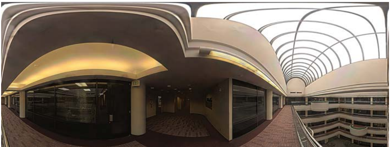
Figure 21: Tone map of the Atrium at the San Ramon, California office of Leica Geosystems. This image is a spherical projection of a panorama assembled from 260 HDR images taken with a ScanStation P40.
