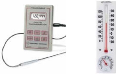
Figure 6: The traceable thermometer on the left is far more expensive than the Acurite® thermometer on the right, who uncertainty is not explicitly given.
