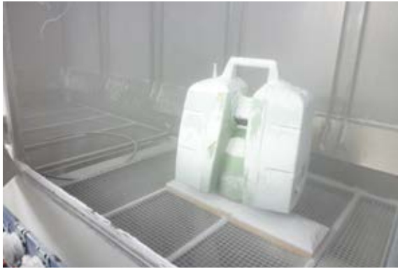
Figure 24: Talcum powder particles are very small and surprisingly invasive, particularly if they have a full day to work their way into the interior of a laser scanner.
