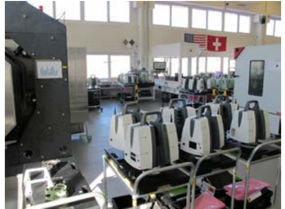
Figure 10: A set of P40 laser scanners awaiting calibration on the manufacturing floor in Widnau, Switzerland.
