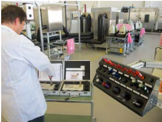
Figure 11: An array of calibrated torque wrenches on the P and C series manufacturing floor at an assembly station, being checked against a calibrated torque reference.
