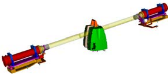
Figure 16: Antipodal placement of the ATEC telescopes allows the telescopes to observe their relative placement, when the scanner is removed. This is a patented twist on the idea of auto-collimation techniques that critically allows for arc second level observation and calibration of laser scanners.
