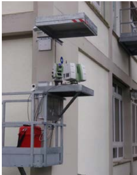
Figure 25: The mounting station for outdoor scanner verification, with a Leica TS30. In the outdoor quality verification test site, a surveying total station is placed next to the laser scanner and collects, in two faces, the coordinates of the targets observed by the scanner at as close to the same time as possible. Clearly the targets are special targets, which dimensionally stable surfaces and mounted with both targets that can be precisely located by the scanner and by the total station.
